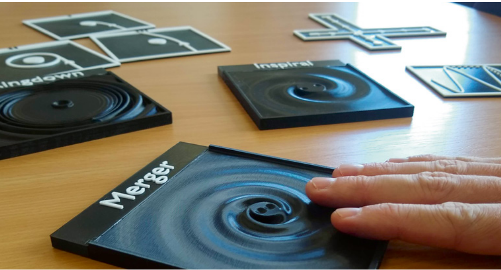
▲ A 3D printed tactile surface showing the inspiral of two black holes and the resulting gravitational waves that the system will produce.
